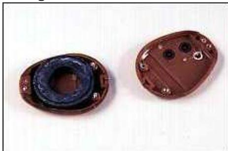
Most of these bits and pieces you can get from an electronics shop. Like all immobilisers, this one shuts down the car's EFI or ignition system. But what's different about this is that if the thief's got your keys (with the remote control attached), he still can't drive away with your car.
