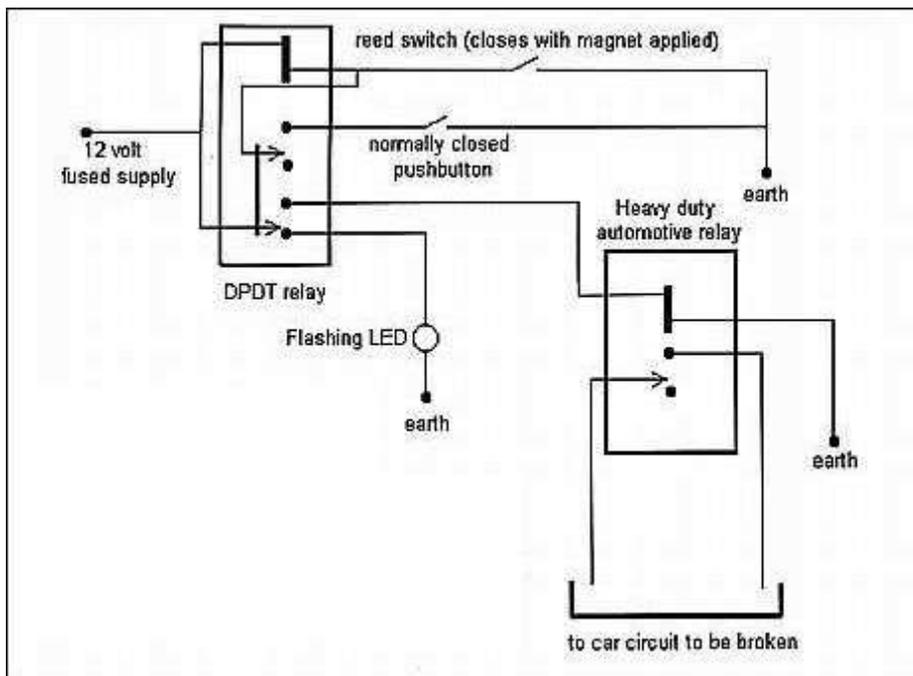
If wiring up a couple of relays doesn't worry you and you can handle a soldering iron and a multimeter, this immobiliser is for you
