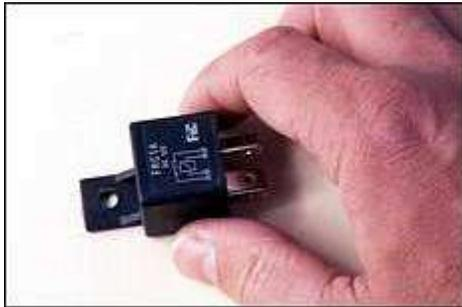
the vital starting circuit. A number of different approaches can be used. In an older car, inserting the relay in the low tension ignition coil power feed will prevent the car starting, as will open-circuiting the ignition key starting signal to the starter motor solenoid. However, if you do the latter, the car can still be "jump started" - not what's wanted!.
