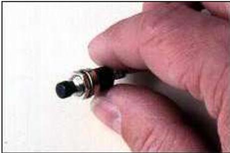
When you want to arm the immobiliser, you press the button. The pushbutton can be in complete view - the thief gains nothing by ripping it out and either disconnecting the wires or bridging them. When you press the button, the on-dash LED starts to flash, indicating the car is now immobilised. It also reminds you to switch off the system when you re-enter the car.
